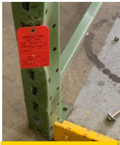
Closed tube damage
