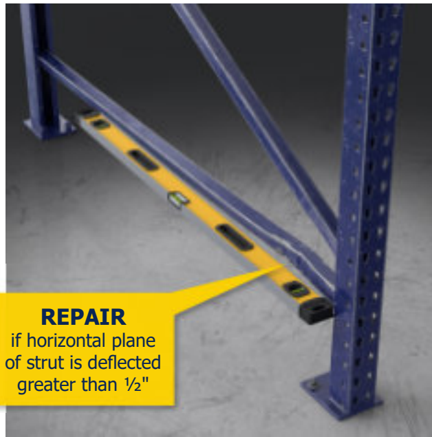
REPAIR if vertical plane of strut is deflected greater than 1/2"
