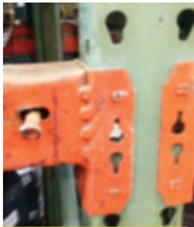
Missing / damaged safety-locks
