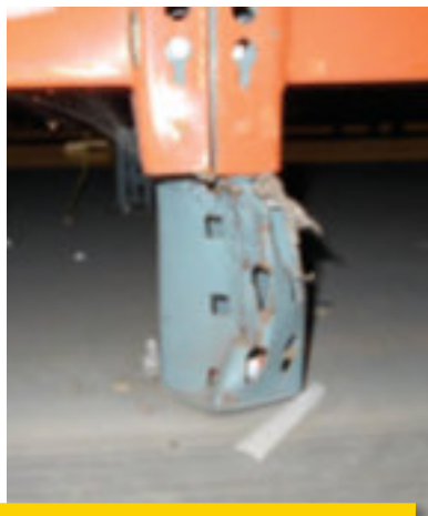
Outrigger damage
